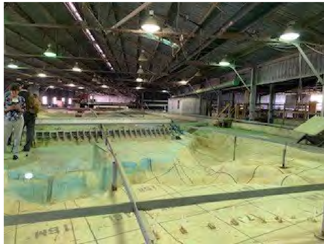
Physical model of The Dalles Spillway
